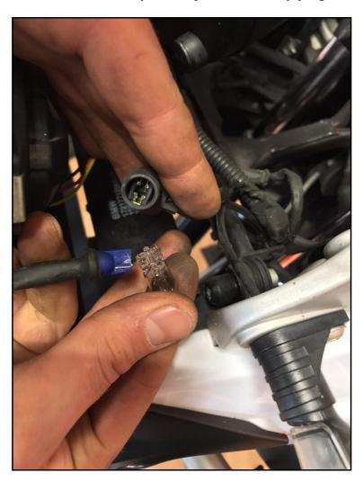
10. Test that the stand warning lamp and Instrumenation day running lighting both function with the ignition in the on position (motor off). If so proceed to Step 11.
