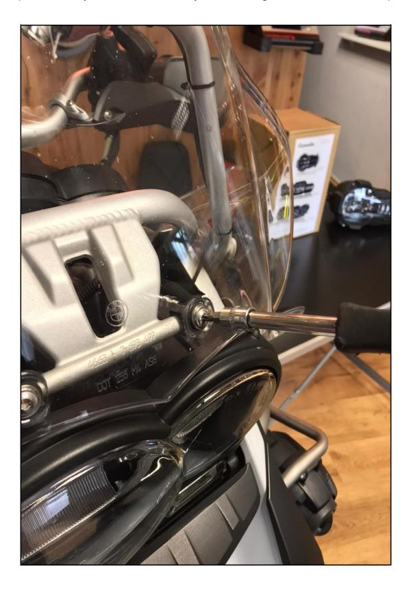
2. Removal of left and right windscreen adjusters. Loosen the adjusters nut with 10mm spanner (or ratchet and socket). With the adjuster nuts removed, the adjusters can be further loosened to gain access to loosen the inside double nut.
