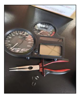
7. Remove the Speedometer from the holder by removing the 3 original Phillips head screws. Install the speedometer to the new headlamp ONLY with the new supplied screws!
