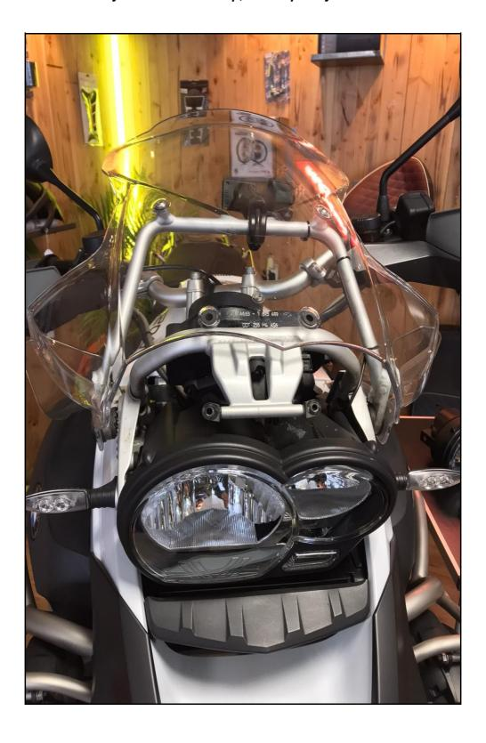
4. Using a Torx 30 driver, remove the headlamp assembly retaining screws left and right.
