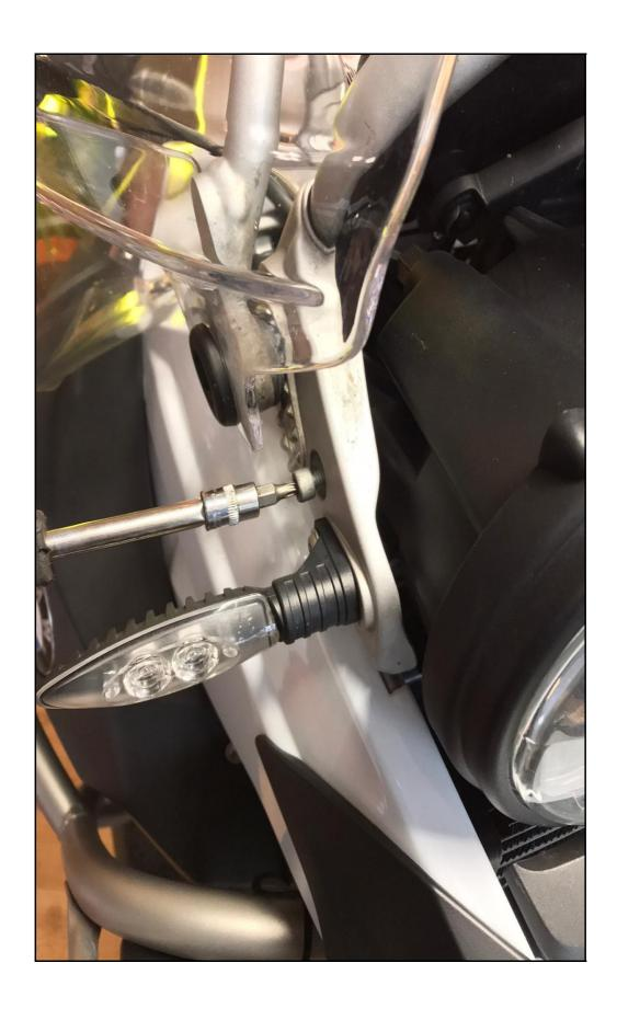
5. Carefully pull headlamp/speedometer assembly forward in the opening. Disconnect wiring connectors for the headlamp and speedometer/instrumentation also the stand warning lamp. then remove the headlamp/speedometer assembly from the motorcycle.
