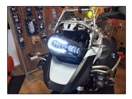
11. Space the headlights with the supplied U-discs/spacers (approx. 2-3 per side / usually left two and right three) and tighten with the original screws.
