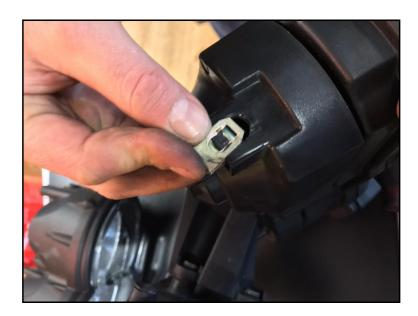
9. Connection of LED headlight to the motorcycle. Connect wiring plugs for the speedometer unit and the LED Headlamp. The stand warning lamp (bulb) is not refitted into the holder, it is replaced by the standlamp plug.
