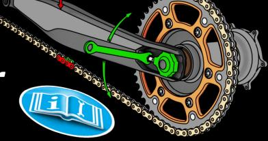
2. Mount the tool with 5. Pull by the handle and secure the bushings on chain's the handle bushing over the chain
