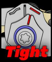
3. Adjust the Chain Slack until the OK marks are aligned
