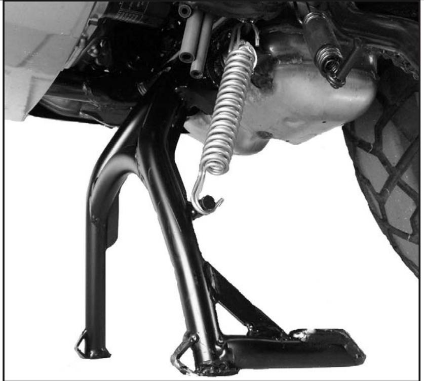
**Please check now the function of your centre stand and control all assembled screw connections for tightness!**
