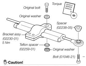
Ensure that there is no clearance problem when turning to the left and the right end positions. Make sure that the steering damper is not used as a stop.
